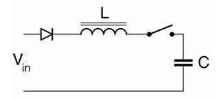
When the switch is closed, the full input voltage is applied across the inductor since the capacitor is initially discharged. Current starts to build up in a sinusoidal fashion and the voltage begins to rise on the capacitor. Once the current has completed a full half cycle, the capacitor is fully charged at twice the input voltage and the series diode prevents discharge back into the power supply. Here's the voltage and current waveforms for some sample component values:
