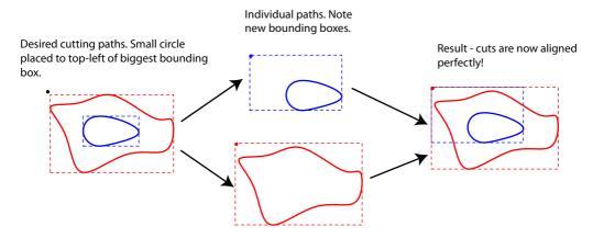
My version of NewlyDraw seems to base things on the top-left of the bounding box, so I place the additional path to the top left. When cutting, make sure this cut is over a piece of scrap material that you don't mind getting fried with the laser.
