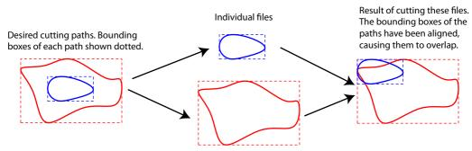
This is obviously no good. NewlyDraw seems to position cut paths based on their bounding box. Therefore, we have to fool it into aligning our paths correctly. We do this by placing a small, additional path, to the left and above the biggest bounding box we have. Viz:
